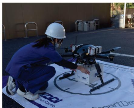
d. Image photo of a transport container on a drone
